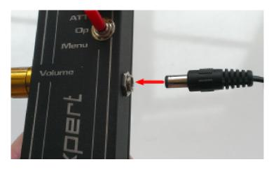
menu, see page 12. The voltage of the fully charged battery is about 8.4 Volts. The battery should be recharged when the voltage has fallen to 7.0 Volts (or anytime earlier). At 6.5 Volts the 'Low Battery Alarm' will sound every 10 Minutes. When it sounds for the first time, you will have enough power left for more than 2 hours of operation. At 6.0 Volts the Receiver will turn off.
