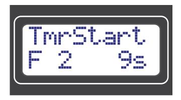
starts transmitting, the time is reset to the value of the fox's transmit time and the count down begins. Press and turn the rotary encoder to select the number of the current fox. The best way to synchronize the fox timer is to turn on the receiver exactly at the moment you start hunting and the first fox starts transmitting. In this case, no additional actions are required.
