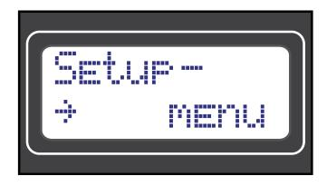
In the setup menu you can change the receiver's main operating parameters. They are: number of foxes, fox transmit time, fox output power, number of frequencies, end-of
