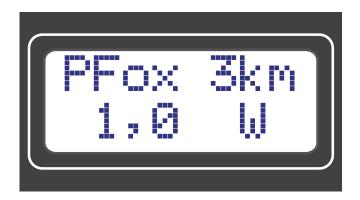
display shows the current attenuation in dB instead of the distance. This mode is not recommended for normal operation. The display shows the estimated distance in the upper right corner. If you know your distance to the fox, like in a 'model event', you can set 'PFox' so that you get the expected distance reading. Recommended setting: '1W'.
