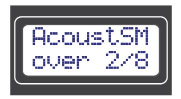
input signal. Switching the acoustic S-Meter on and off is done by clicking the Encoder in the main operating mode.
