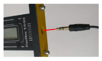
disconnect the headphones and push the Encoder for several seconds until the display goes off.
