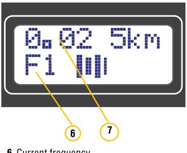
frequency number will be indicated by the number after the letter "F" in the lower left corner of the screen. The length of the scale of the signal level meter will decrease.
