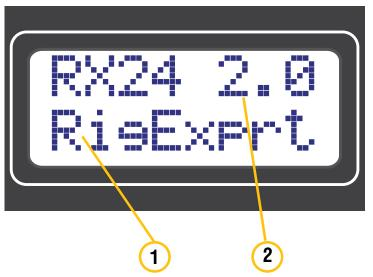
After power ON, a start text and software version information are briefly displayed on the screen. Then the receiver goes to the main operation mode. The start text can be changed to your name or callsign in the Calibration menu, see page 22.
