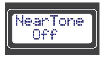
to select the distance for the single/triple tone warning from 300m/70m to 30m/5m, or select 'Off'. Recommended setting: 'Off'.
