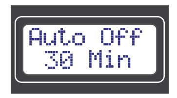
receiver will go off. Select menu item 'Auto Off' and push+turn the Encoder to set the time from 10 to 70 minutes, or to 0 for no auto-off. Recommended setting: '30 Min'.
